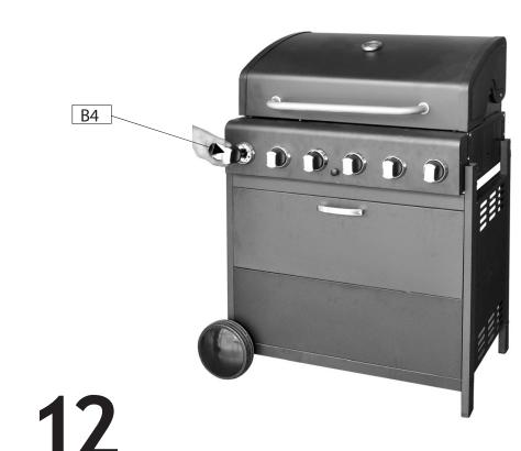
Press the knobs (B4)onto valve stems as shown.
