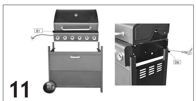
Carefully place the Barbecue Body (B1) onto the cabinet structure and fix using M6x40 Bolts (D6x8pcs) as shown.
